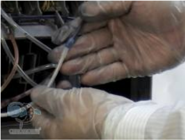
07. Connecting CFS's tube with ink tube of printer.
