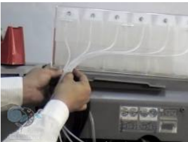
11. Clamping 6 tube by clip provided and taping the gap of clip by tape.
