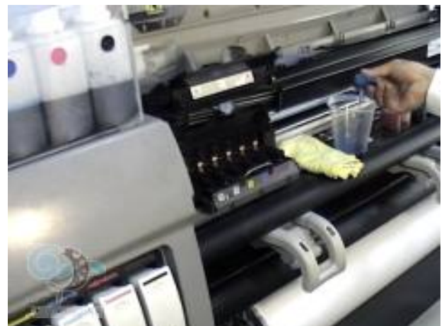
24. Drain the all ink of vacuum bottle.
