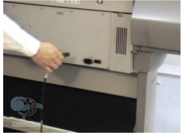
02. Power down printer, remove the power cable of printer.
