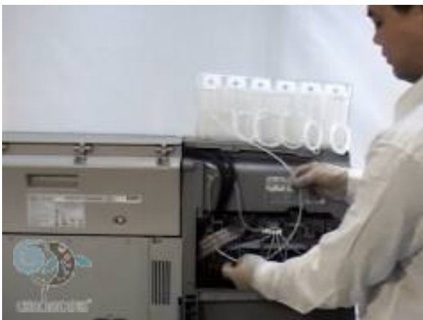
05. Loose the tube of CFS.
