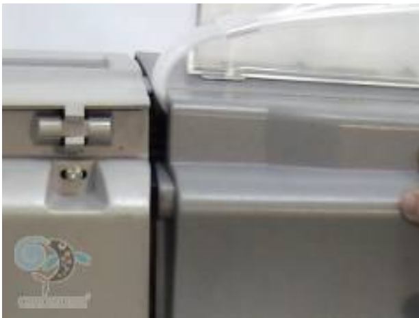
15. Try to open the front cover, check if it will jam with tube of CFS.
