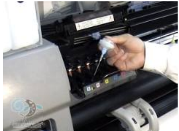
22. Use vacuum bottle to draw out remain ink which in tube of printer.
