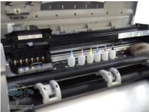
21. Take out all printhead, prepare vacuum bottle provided.
