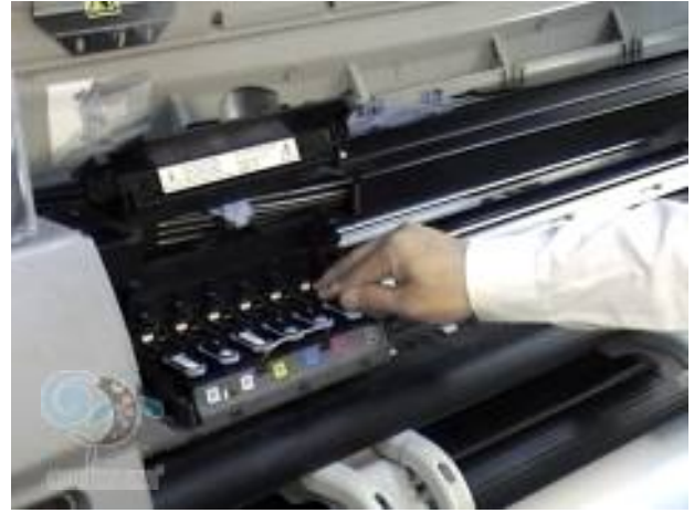
26. Put back printhead in carriage.
