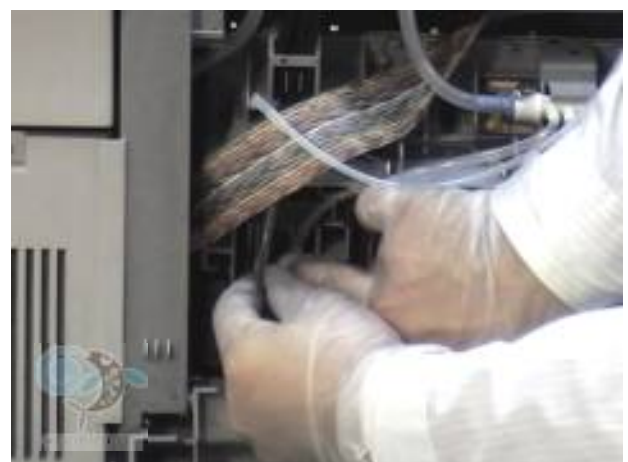
06. Pull out the ink tube of printer.
