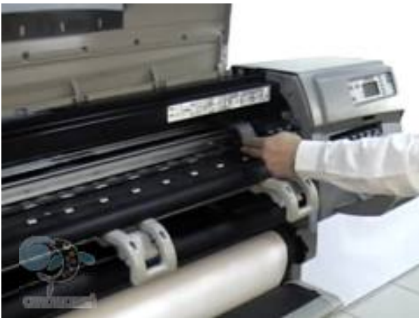
27. Push back the printhead carriage.
