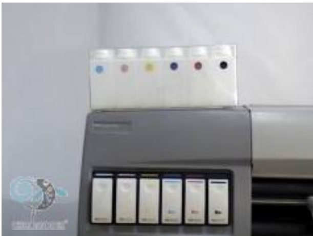
03. Place CFS on the printer platform.
