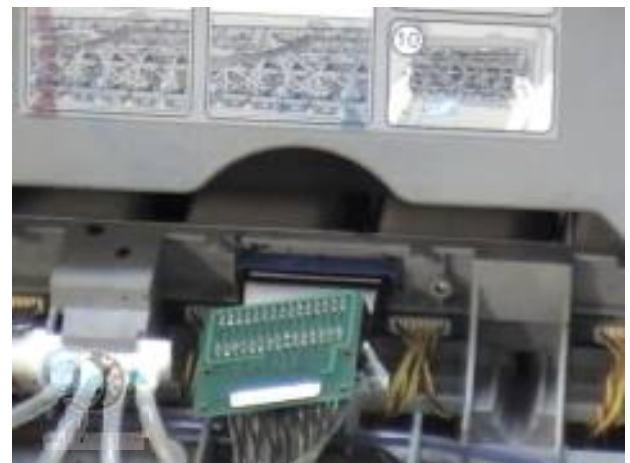
18. Insert data cord into solution card, then insert solution card into data socket of printer.
