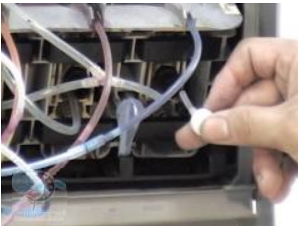
09. Insert Stopper into ink outlet of printer.
