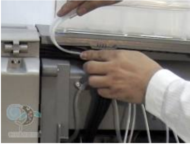
13. Bend the two clip and put them into the gap of printer.
