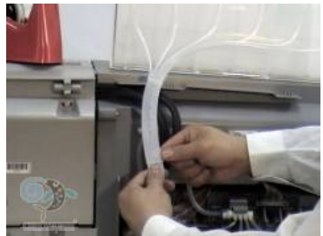
12. Clamping and taping again below about 15cm of the first clip.
