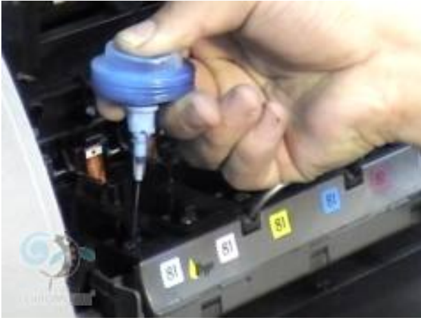
25. Use vacuum bottle again to draw out remains air in the tube of printer.
